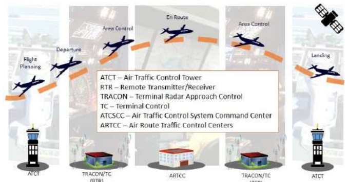
Figure 1. Facilities of an Air Traffic Control System
