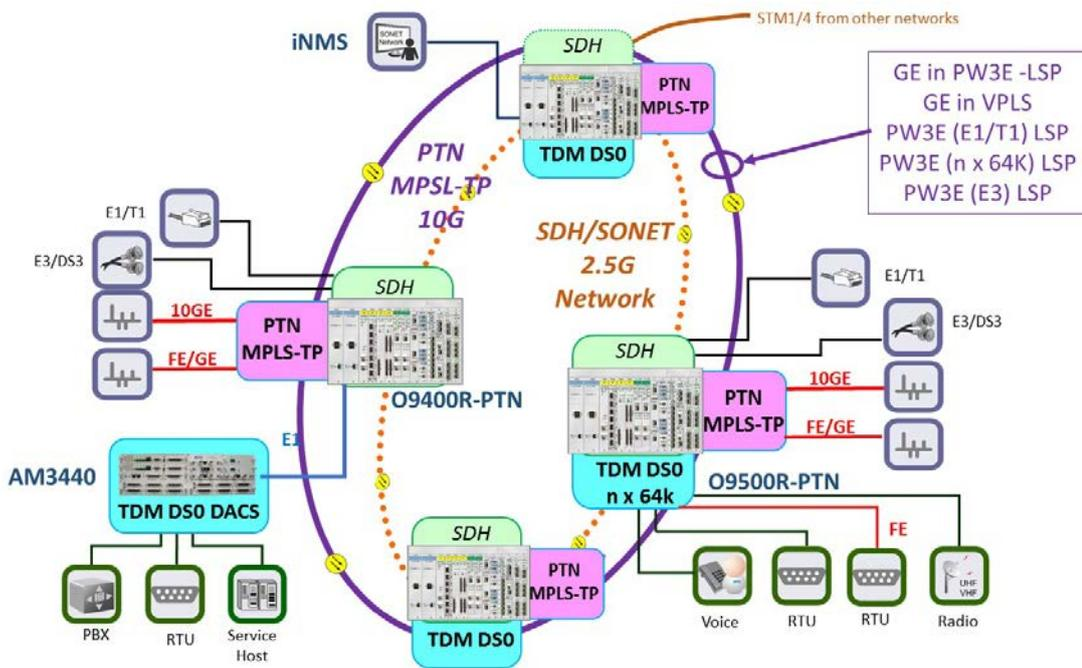
Figure 1-5 PTN MPLS-TP infrastructure to transport Ethernet, Multiservice TDM and eventually SDH links
