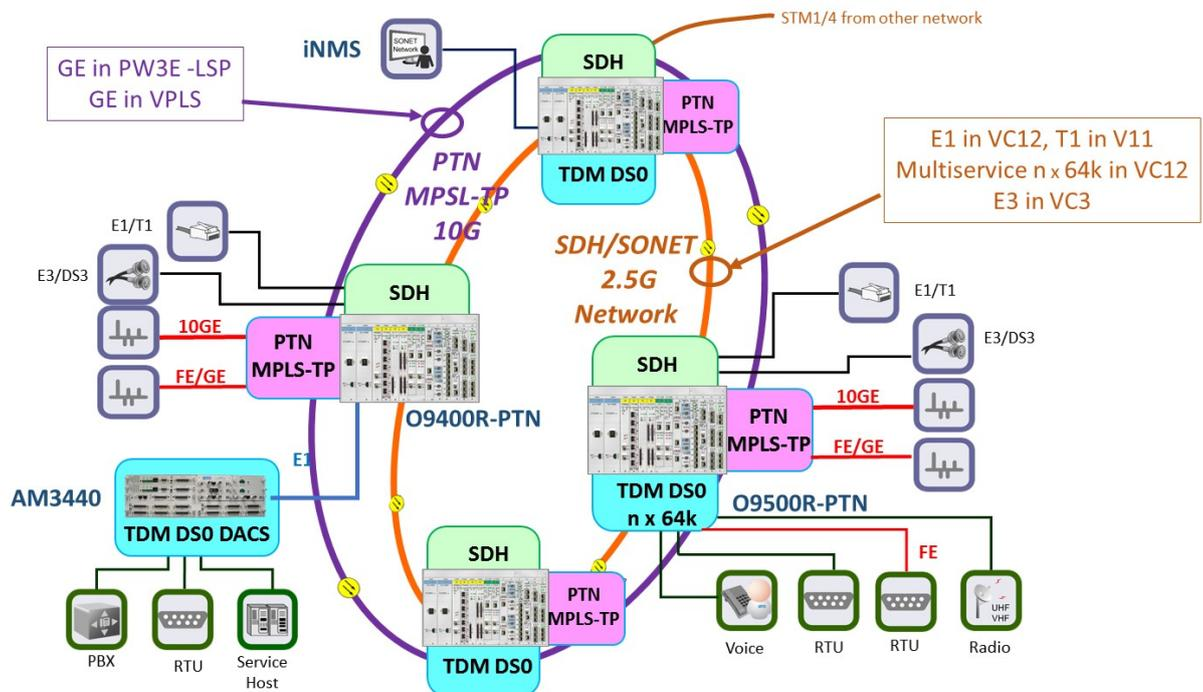
Figure 1-3 Standard SDH/SONET for Multiservice transport and Ethernet SCADA and PTN MPLS-TP for Ethernet transport infrastructure
