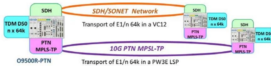
Figure 1-1 E1 TDM transport over SDH/SONET and over PTN MPLS-TP
