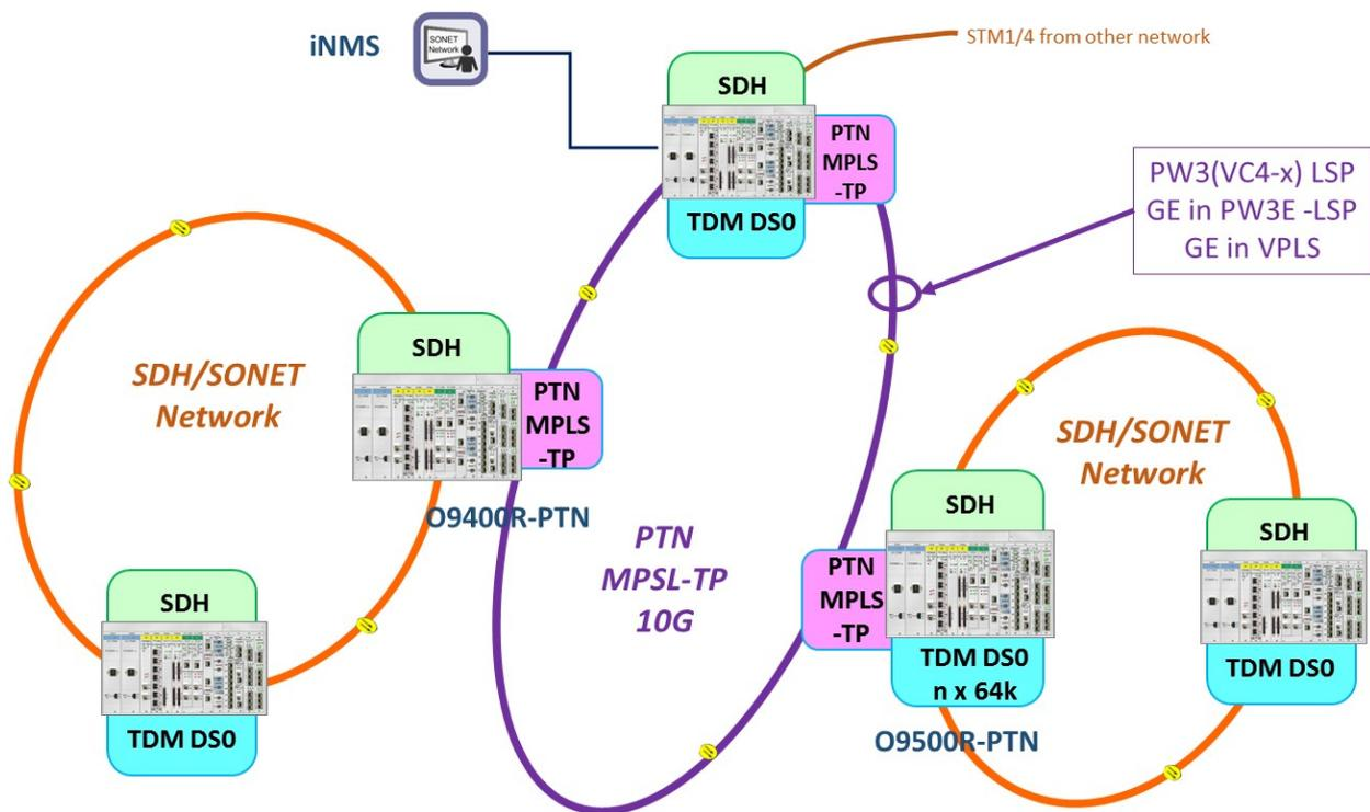
Figure 1-4 Standard SDH/Sonet for Multiservice transport and Ethernet SCADA crossing PTN MPLS-TP infrastructure
